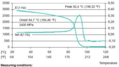
Sample thickness: 2 mm Heat rate: 2 K/min
