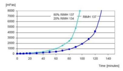
Measuring conditions: Temperature: 40°C (104 °F); measuring gap 0,2 mm
